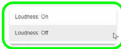
Selecting "loudness on" will boost low & high frequency response at low volume. The curve will be active until half volume where it will be completely flat
