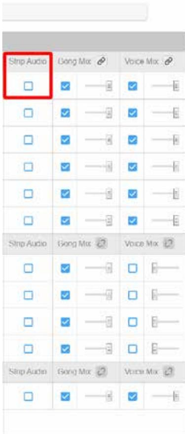
The strip audio feature allows you to remove all audio from each analog output while leaving all factory gongs, handsfree audio and audible navigation prompts. This feature is used commonly with an external DSP that allows digital Toslink and analog inputs to mix. An example would be using the Toslink set to “front fading” to provide audio to the front speakers and using the analog front channels to provide the mix in of the factory gongs, handsfree and audible navigation prompts.
