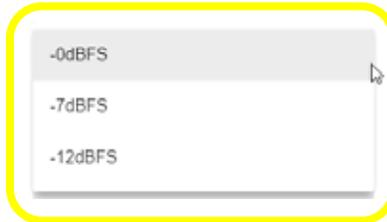
Global output adjustments: At -0dBFS the unit provide a full-scale output. At full volume, minor adjustments of the factory bass or treble can produce digital clipping. With the bass and treble set to neutral the unit will not clip at full volume. -7dB provides the ability to adjust the factory tone controls moderately without clipping at full volume and -12dB allows for maximum adjustment of the OEM controls without clipping.
