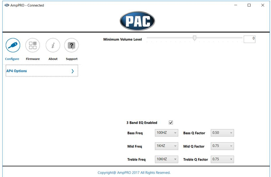
**PLEASE NOTE:** These settings can be adjusted with the module installed in the vehicle or on the bench. However, it is recommended to make the adjustments with the module installed, and the factory radio on so that the changes can be heard.
