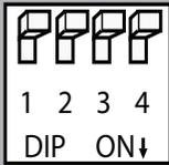
Set DIP switches to the ON position to activate the corresponding features.
