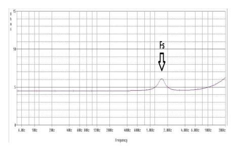
Figure 2, Impedance curve of a typical 4 ohm, 1" tweeter. Notice the  $f_{\rm S}$  at 1.59 kHz
