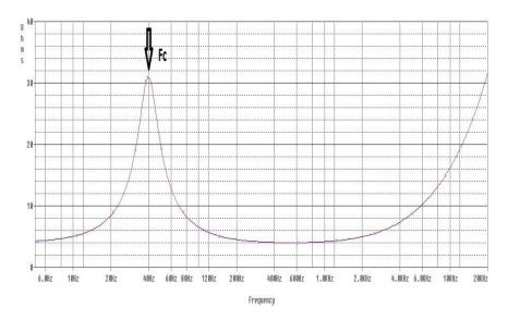
Figure 3,  $f_{\text{C}}$  of a single 4 ohm, 15 inch subwoofer in a 2 cubic feet sealed box.
