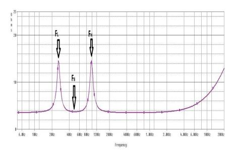
Figure 6, the impedance curve of a single 4 ohm voice coil subwoofer in a single reflex bandpass enclosure (4th order). Bandwidth is approx. 30-90~Hz
