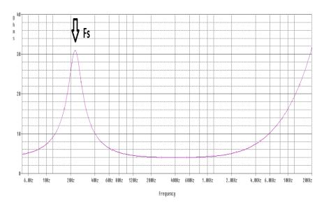
Figure 1, Impedance curve of a single 4 ohm voice coil, 15 inch subwoofer. Notice the  $f_{\rm S}$  at 24 Hz.
